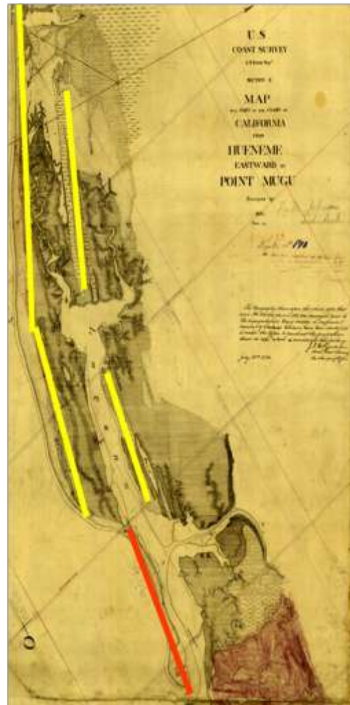
Figure 4. Series of barrier sand spits generating the prograding shoreline and forming much of the space of Mugu Lagoon (ca. 1860). Note the stable sand spits (yellow bars) apparently formed by a succession of longshore “trapping” events. Note also the thin spit (red bar) historically observed to undergo cycles of mouth migration, closure, and breaching as supported by observation, successive mapping, and air photography (see Warne 1971). In addition, the older Holocene inland spit is cross-cut by an outflow channel contributing to the estuary space. This cross cutting feature was apparently associated with flood distributary behavior of the Santa Clara River.
