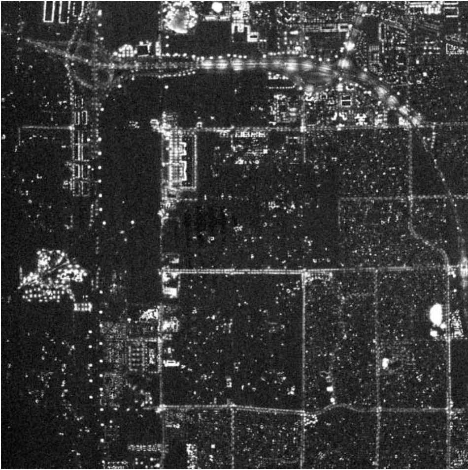
Figure 5. Airborne night-time lights imagery at 1.5 m resolution covering a portion of Las Vegas, Nevada. Imagery acquired from NASA's ER-2 flown at 13.7 km above the Earth with a Cirrus DCS digital camera.
